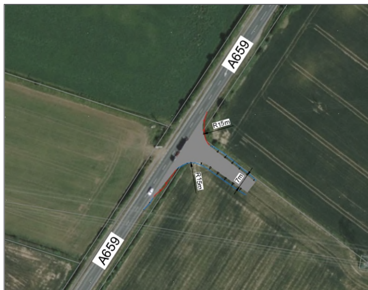
Figure 10: Upgraded Northern Access Bellmouth
