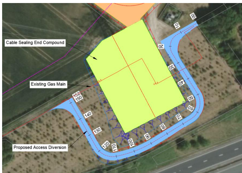
Figure 11: Existing Gas Main Interaction
