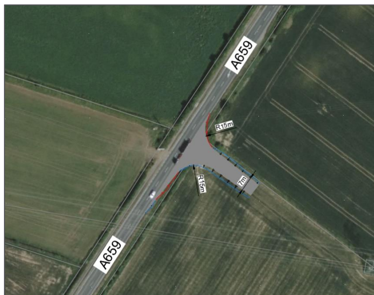
Figure 10: Upgraded Northern Access Bellmouth
